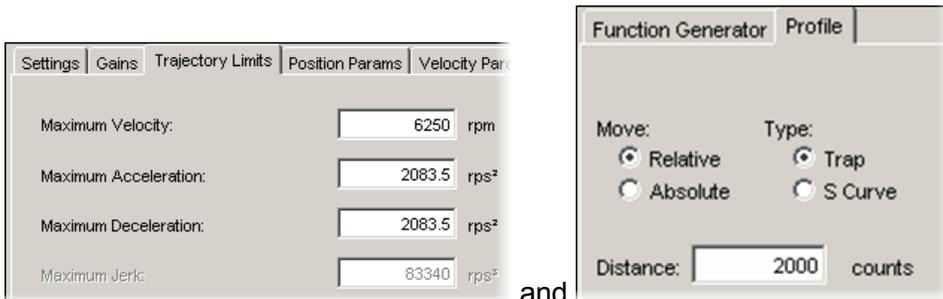
Set up a trapezoidal profile by setting the trajectory limits and distance. See table:
