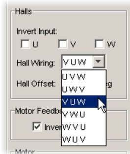
If the red indicator transition leads or lags behind the centered needle by more than 30 degrees, then try adjusting the *Hall Offset* in +/- 30 degree increments:
