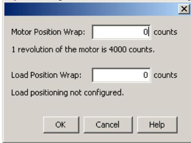
**4** Change/verify the position wrap parameters as needed. Set both values to zero to disable position wrapping. Note that the changes do not take effect until **OK** is pressed. For more information about this feature, see [Position Wrap \(p. 114\)](#).
