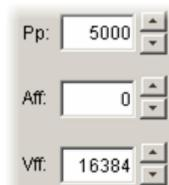
Adjust position proportional gain (Pp) to minimize following error:
