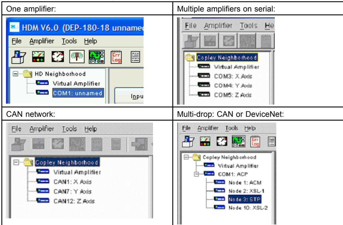
When there is only one amplifier available for connection, the software will connect automatically on startup.
