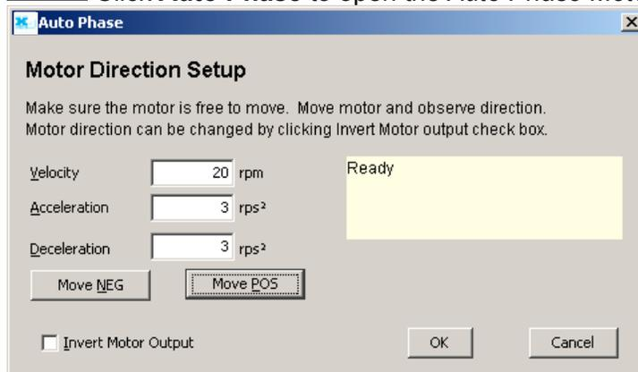
3 Hold down **Move POS** to move the motor in the direction considered positive, and observe the direction of movement.
