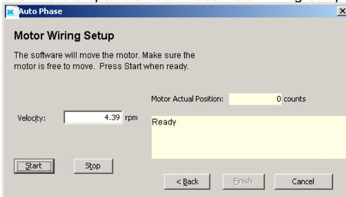
6 Click **Start** to begin motor wiring setup with default values. After successful motor wiring setup, the message “Test Complete” appears.
