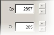
On the *Gains* tab, adjust current loop proportional gain ( $C_p$ ):
