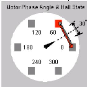
If the needle and Hall states do not track properly, use the *Hall Wiring* list box and/or Invert Input options (shown below) to swap the amplifier's Hall wire configuration.
