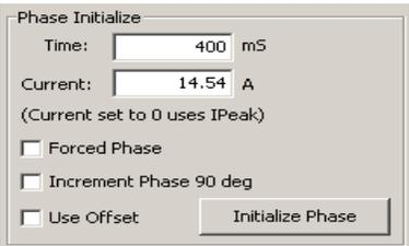
If the phasing function fails (for instance, message “Phase Initialized” is not displayed, or if a phasing fault is indicated) adjust the phase initialization settings described below and try Step 4 (**Initialize Phase**) again.
