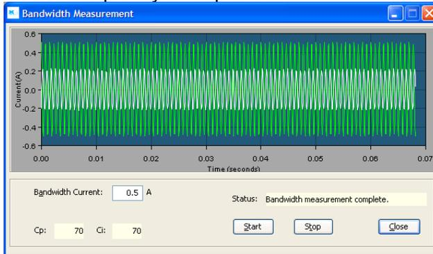
Displays the results: a set of  $C_p$  and  $C_i$  alternatives, and the bandwidth measured using the high  $C_p$  and  $C_i$  values.
