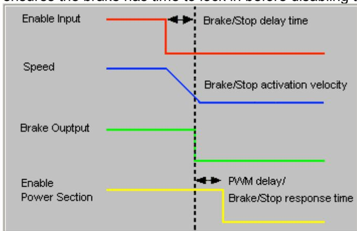
This sequence is not available in the current mode of operation. Instead, in current mode, the amplifier output turns off and the brake output activates immediately when the disable command is received.
