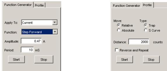
The **Start** button starts the function or profile generator. The **Stop** button stops the generator and aborts any profiles in progress.
