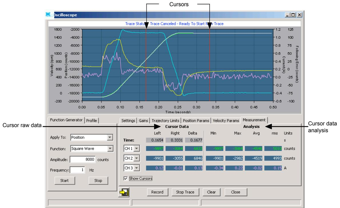
When **Show Cursors** is not set, the Cursor Data fields are inactive and the Analysis fields show calculations based on data from the entire trace cycle.
