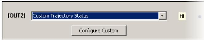
Choose **Custom Trajectory Status** for an output and then click **Configure Custom** to open the *Trajectory Status Configuration* screen.
