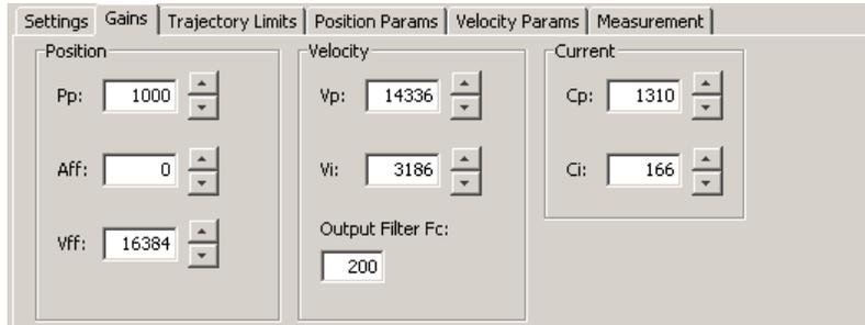
Note that the parameters represented on these tabs can also be accessed through the screens used to configure the control loops and the digital position input. Changing a value in the Scope tool automatically updates the value on the other screens where it appears, and vice versa.
