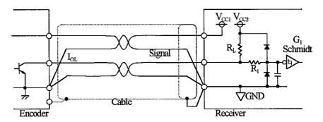
(1) Set the pull-up resistance (RL) with the following equation so that IoL is 5~20mA.
