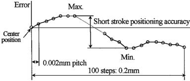
Short stroke positioning accuracy = Maximum error - Minimum error
