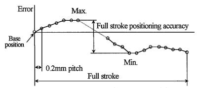
Full stroke positioning accuracy = Maximum error – Minimum error
