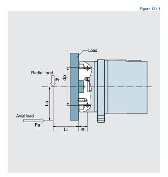
**■** How to calculate the average load (Average radial load, average axial load, average output rotational frequency)
