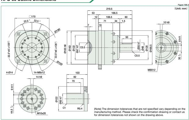
Only primary dimensions are shown in the drawings below. Refer to the confirmation drawing for detailed dimensions. For the specifications of the input side bearing, refer to page 133.
