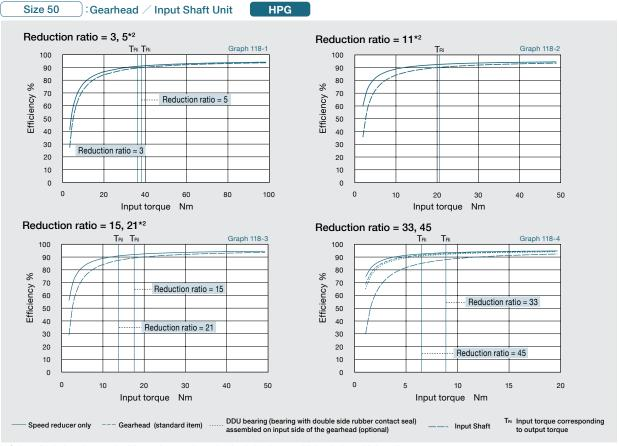
\*2 Only one line is shown because the difference between the gearhead and a bearing assembled on the input side is small.
