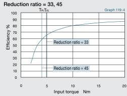
$T_{\mbox{\tiny Ri}}$  Input torque corresponding to output torque
