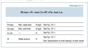
How to calculate the radial load coefficient and the axial load coefficient
