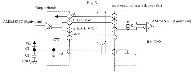
Voltage strength of capacitor C1,C2:50V
